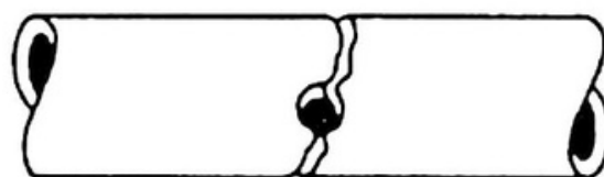
Cracked pipe after hot tap
