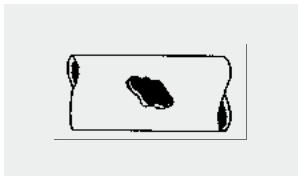
Pin holes in asbestos-cement, cast iron, steel and plastic pipes
